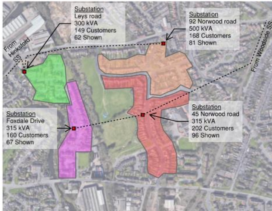
Figure 13 - Assumed substation zoning
